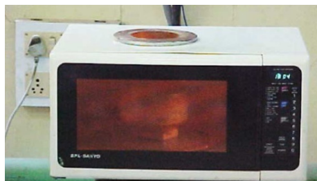
Fig. 1. Modified domestic microwave oven used for synthesis of SrLa y Fe 12-x-y Cr x O 19 .
